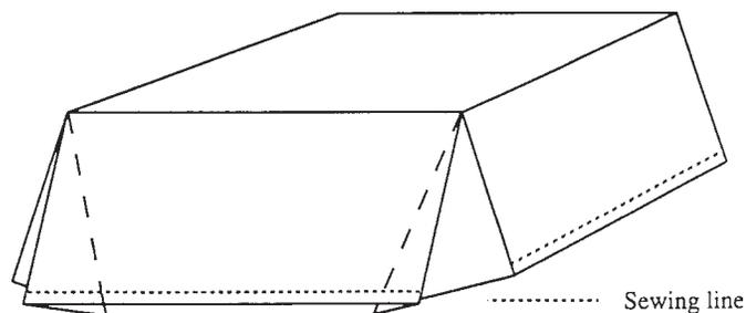
FIG. 5 Folding of Fabric for Loose Filling Materials
